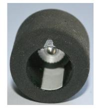
Now cut a small piece of adhesive tape and place inside the wheel, exactly opposite the mark.
